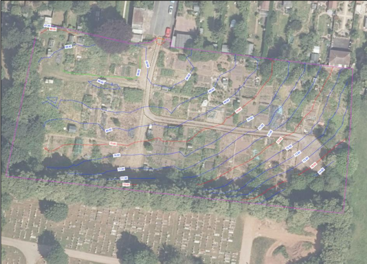
Figure 8. Levels survey results (0.50 m contours).
