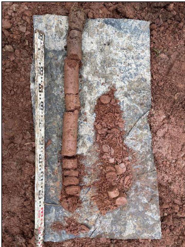
Figure 39. Window sampling cores from TP3.
