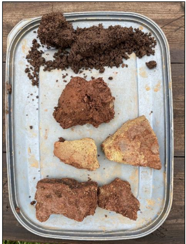
Figure 40. Soil samples from 0.1 m to 2.2 m – TP3.
