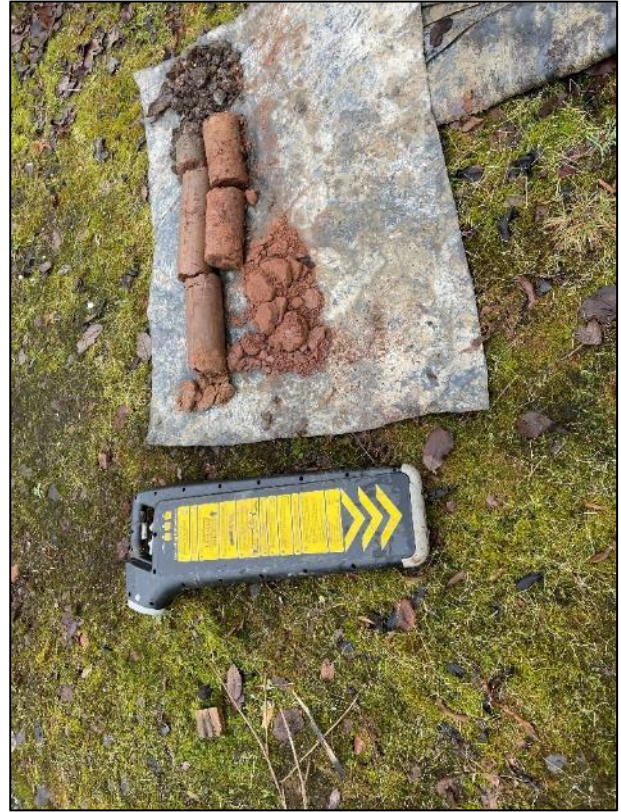
Figure 28. Window sampling cores from TP1.
