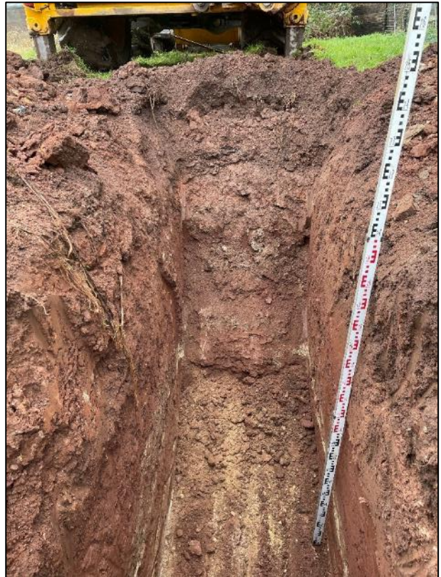
Figure 38. Grey SANDSTONE to 2.00 m over hard red SANDSTONE – TP3.
