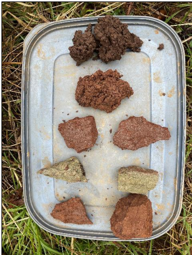
Figure 33. Soil samples from 0.1 m to 2.9 m – TP2.
