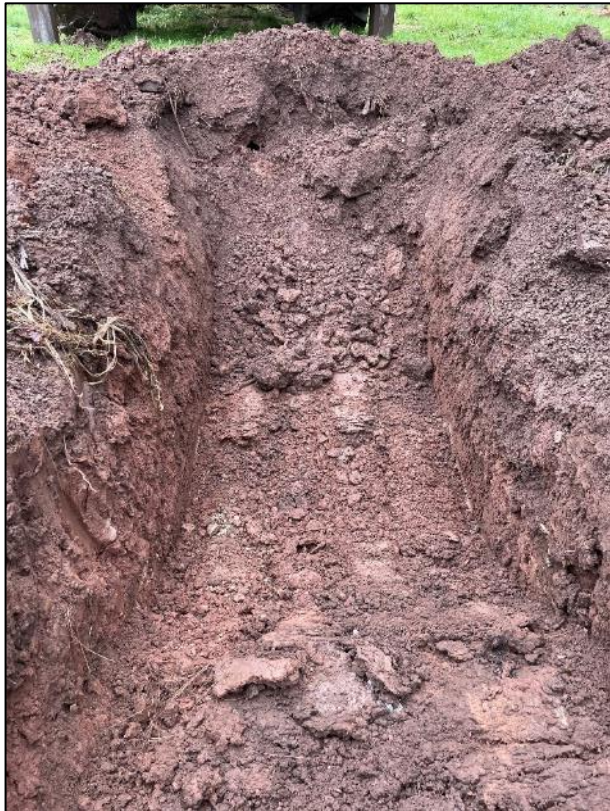
Figure 37. 0.25 m of brown CLAY LOAM topsoil over red CLAY LOAM subsoil (mudstone) to 1.80 m – TP3.
