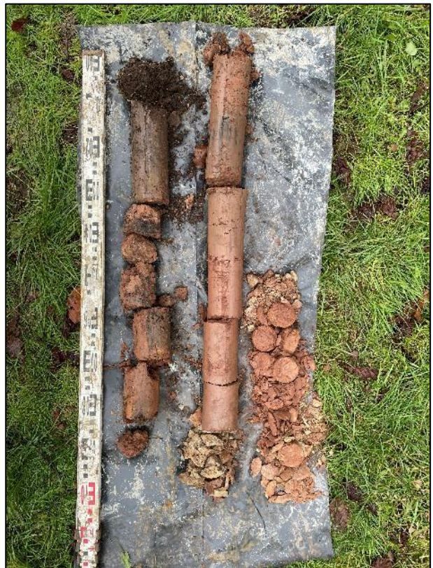
Figure 34. Window sampling cores from TP2.
